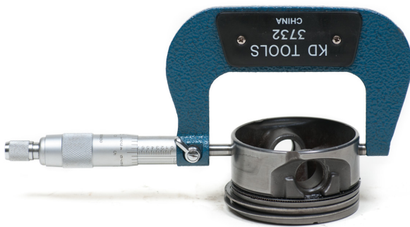
Figure 2—Measuring a piston
