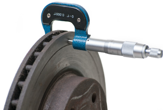
Figure 3—Measuring a brake rotor
