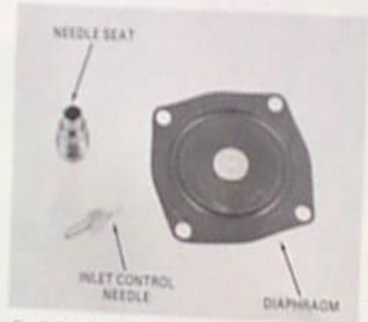
Fig. 5-26. A diaphragm, control needle, and needle seat used in a diaphragm carburetor system. (Deere & Co.)
